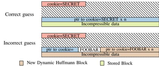
Fig. 10: Incorrect guesses with the corner case discovered by Comprezzor lead to a dynamic Huffman block creation for the partially-compressible data that is slow to decompress.
