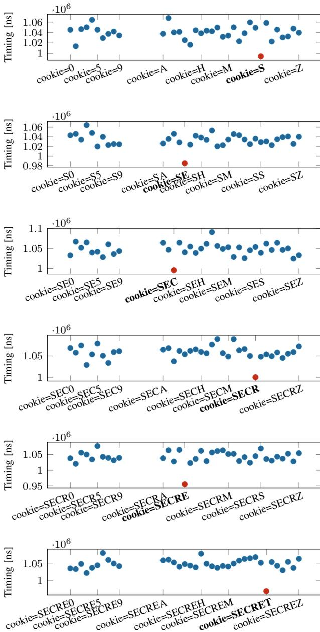
Fig. 11: Bitwise leakage of the secret (S,E,C,R,E,T) from PHP-Memcached. In each plot, the lowest timing (shown in red) indicates the correct guess. The standard error is below 1% for all guesses.
