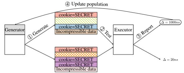
Fig. 4: *Comprezzor* generates memory layouts with different entropy, input size, and secret alignment, leading to high-latency decompression times. Every iteration, samples with the highest latency difference are used as input to generate newer layouts.
