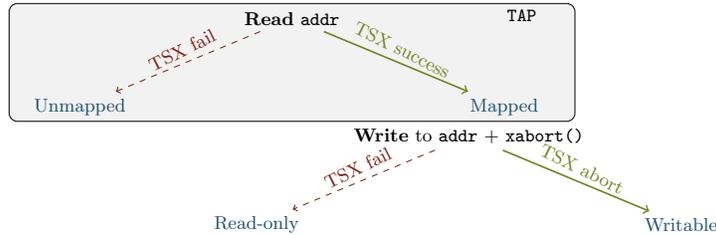
**Fig. 4: *CLAW* exploits that memory writes in TSX are only visible to the outside of a transaction if it succeeds, and that TSX distinguishes between implicit and explicit aborts. Thus, the return value of TSX after writing to an address and explicitly aborting determines whether the memory location is writable without changing it.**
