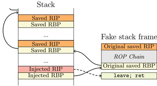
**Fig. 3: To divert the control flow without interfering with legitimate stack frames, the attacker injects a new stack frame. The new stack frame can be used for arbitrary code-reuse attacks without leaving any traces in stack frames of other functions.**
