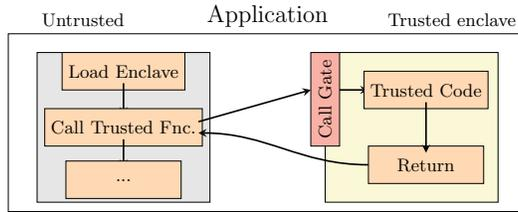
**Fig. 1: In the SGX model, applications consist of an untrusted host application and a trusted enclave. The hardware prevents any direct access to the enclave code or data. The untrusted part uses the EENTER instruction to call enclave functions that are exposed by the enclave.**
